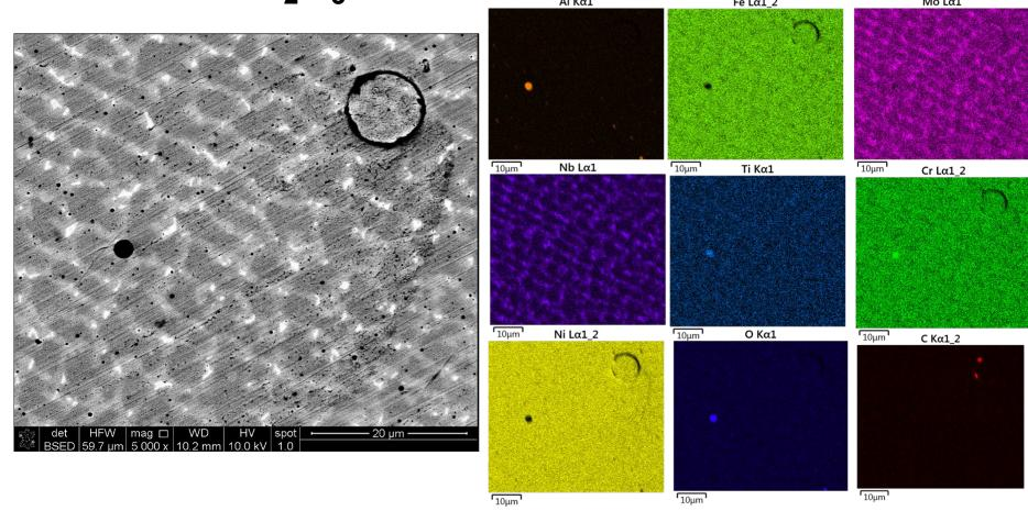
EDS analysis shows the increased presence of aluminum, chromium, titanium, and oxygen in particles of SEM image. This shows the chemical reaction of the chromia oxide in the 718 alloy and the even dispersion of oxide particles into the nickel matrix.
